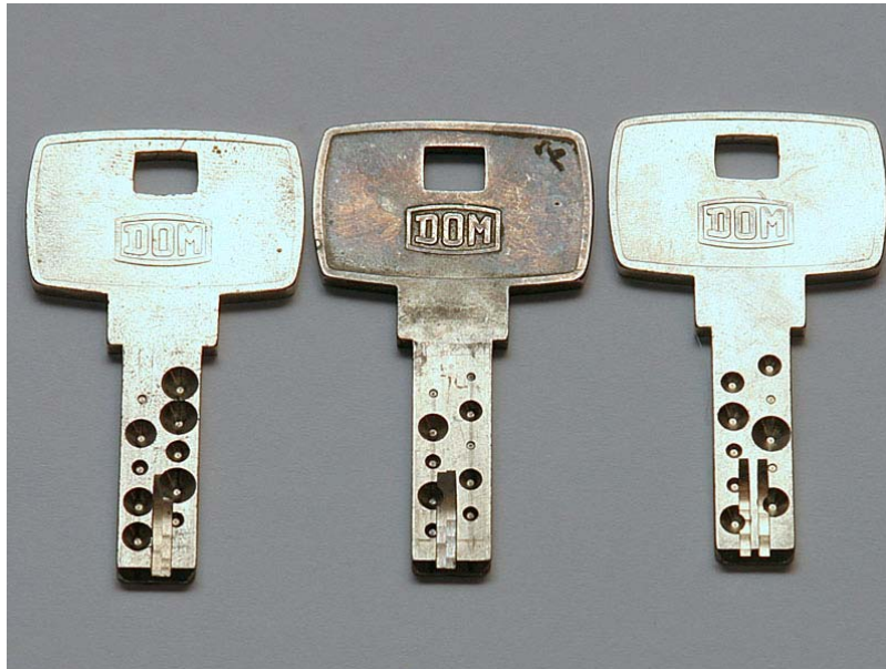
3 different old ix-10 key profiles with extra grooves on the left and right side of the key (not visible).
