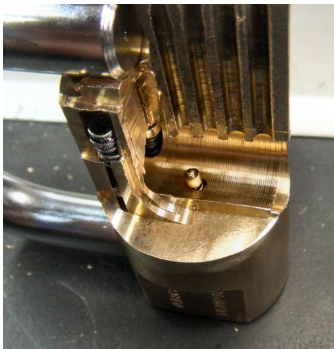
Figure 7: Viro cutaway showing the detent.
