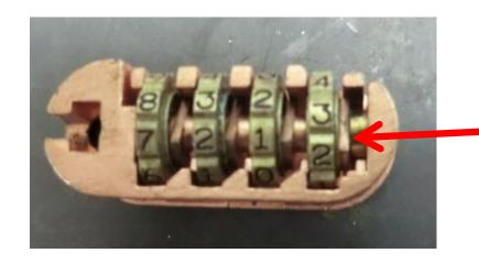
Each wheel has a flat spot. I have these aligned so you can see them clearly. Notice the locking pawl activator is in the "up" position.
