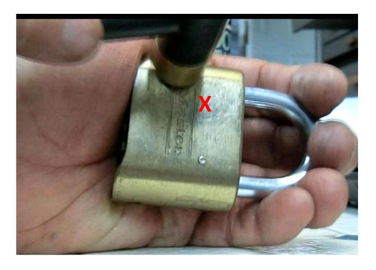
Use a brass or hard plastic hammer. Don't use steel because it will seriously mar the lock. Give the lock 20-30 whacks as close to the "X" as you can. The pin will begin to work itself out. In the photo my pin is already backing itself out. Plastic hammers will take more whacks but do almost no damage at all.
