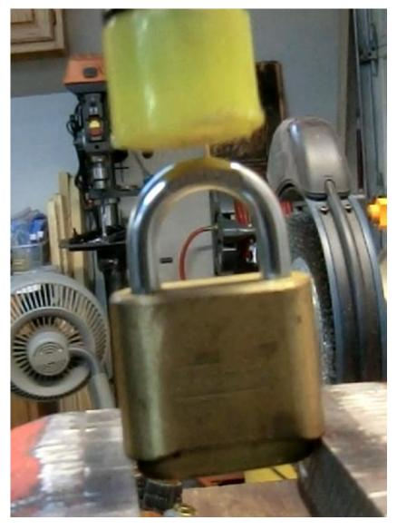
Usually the guts just fall out of the brass body. If not, put it in your vise with the jaws lined up with the brass body. Gently tap the hasp and the guts will fall out. You can see mine coming out.
