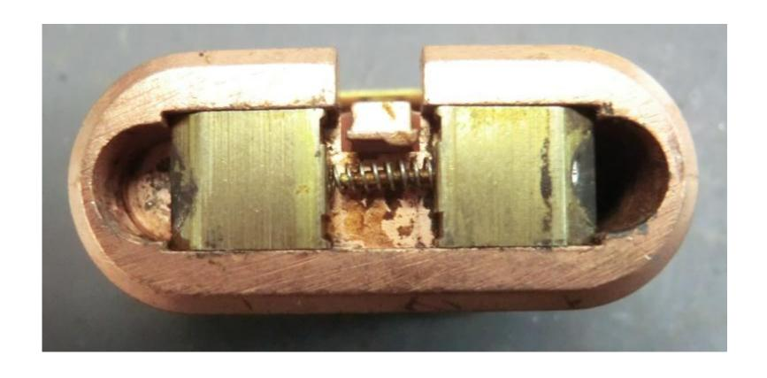
On the top, put your locking pawls back in. Leave the lock sitting upright with the pawls on top – it'll be easier to reassemble that way.
