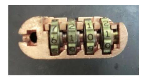
Turn your wheels until they are under the locking pawl activators and it moves down. Read your combination. Write it down. In this case it is 6101.
