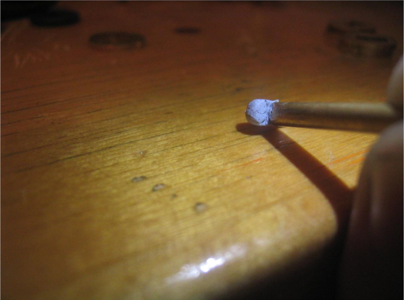
After the impression has been made, the tool is carefully turned 90 degrees to where it came from and then carefully removed from the lock. The result should be something like in the above photograph. It shows a number 6 impressed as a mirror image on the Blu-Tack. As all the numbers 1, 2, 3, 4, 5 and 6 are slightly different from each other, they can be easily recognised from the impression mark even if the impression is partial or bends a little while removing the tool from the lock.
