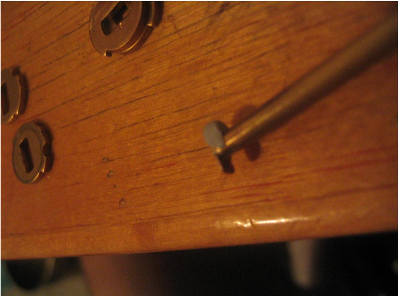
In the above photograph can be seen that I've stuffed the Blu-Tack around pick tools end on the "user" side. I only applied it to the other part of the pick tools end, but it can be applied to both sides. This way it'll give stability in the lock and you don't have to think about at which side of the detainer disc the stamped number was.
