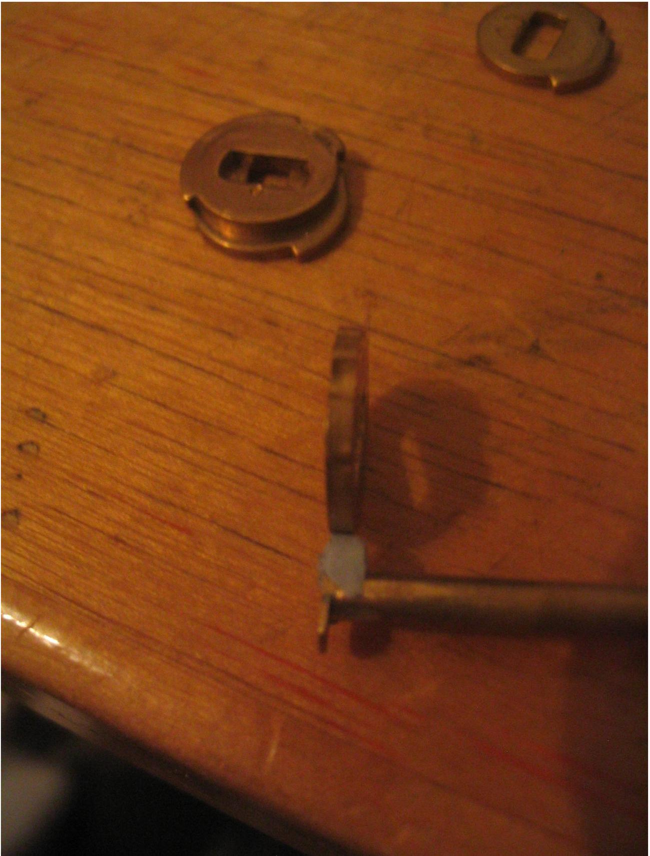
The thickness of the Blu-Tack plus the pick tools end should not exceed that of the detainer disc. This is because the pick tools end still has to have room to turn in the lock. In the above photograph the Blu-Tack is a little too thick.
