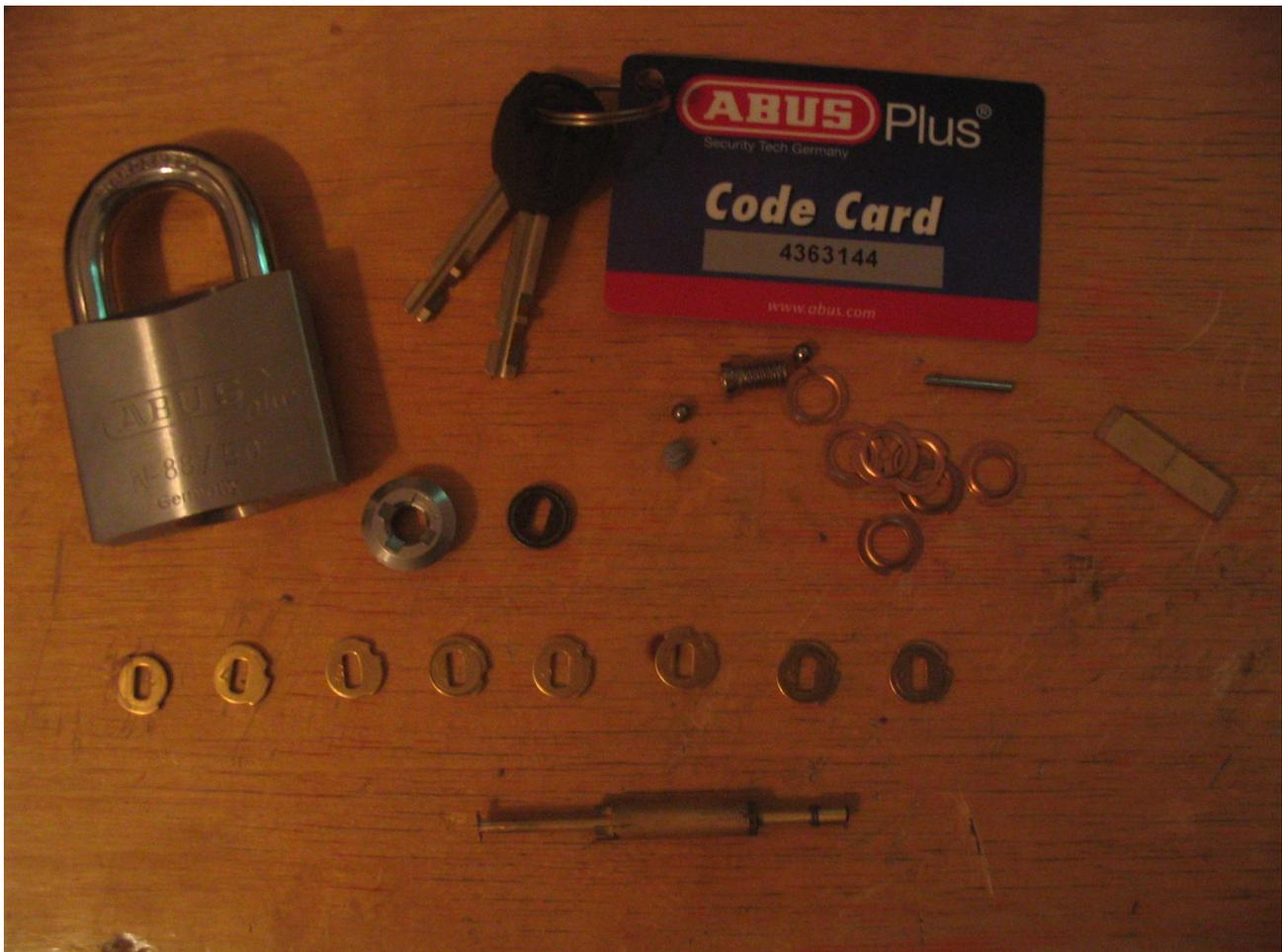
In the above picture can be seen the Abus 88/50 padlock that costs about 20-25 Euros. It is equipped with the Abus Plus cylinder, that is a rotating detainer disc style cylinder. The code card shows a number sequence 4363144. The code corresponds to the cuts in the key such that number 6 cut is a no-cut and number 1 is a fully cut. The numbers correspond to the cuts from bow to tip.
