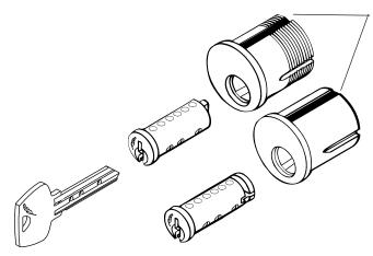
Top Loading of Cylinders allows for easier field pinning (since May 2008)
